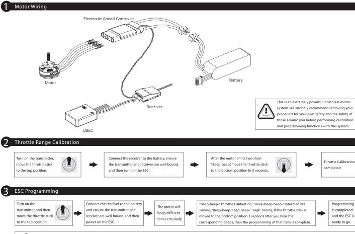
Generally speaking, intermediate timing is applicable to most motors and it brings higher efficiency but less heat to the motors and speed controllers. High timing can increase the RPM of the motor, but it also increases the motor temperature. Please perform a test flight on the ground and ensure everything is functioning properly first, then fly your aircraft into the sky.
